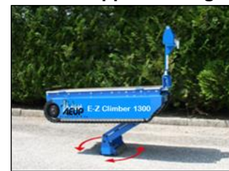
Roller rotation, zero-turning, fine-tune approach angle
